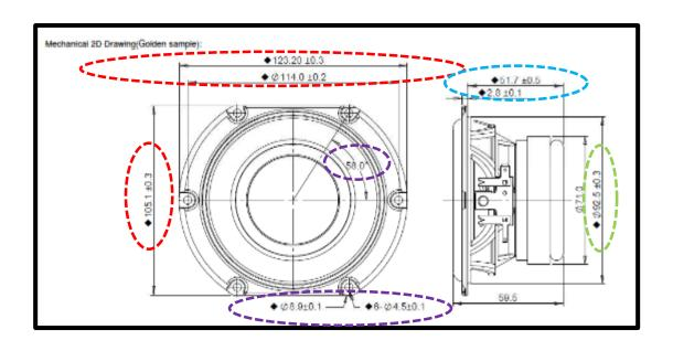
The mechanical drawings shown on specification sheets (see picture above) will show dimensions typically relating:
