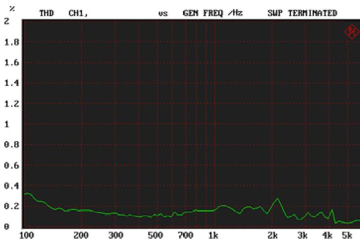
**Mid-band distortion (Epos Encore 50 loudspeaker).**
