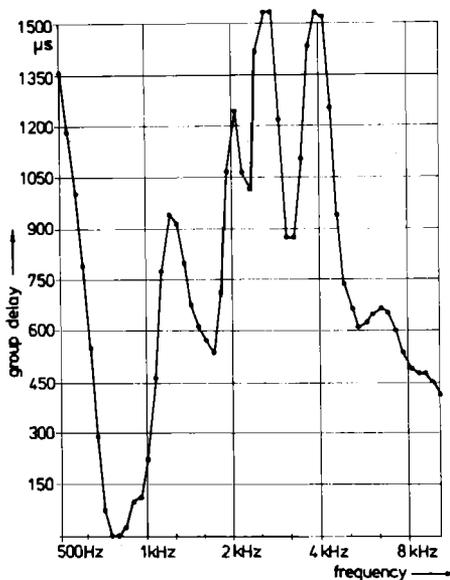
FIG. 4. Group delay caused by all-pass contents: noncommercial bass reflex box with exponential horn (approximately 450 dm<sup>3</sup>). Pickup point on the axis, distance 3 m, anechoic chamber.
