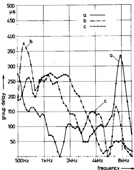
FIG. 3. Group delay caused by all-pass contents: (a) Philips 9710 M loudspeaker in 16 dm<sup>3</sup> closed box, (b) Heco B 180/M closed box (approximately 14 dm<sup>3</sup>), (c) Isophon KSB 12/8 closed box (approximately 6 dm<sup>3</sup>). Pickup point on the axis, distance 1 m, anechoic chamber.
