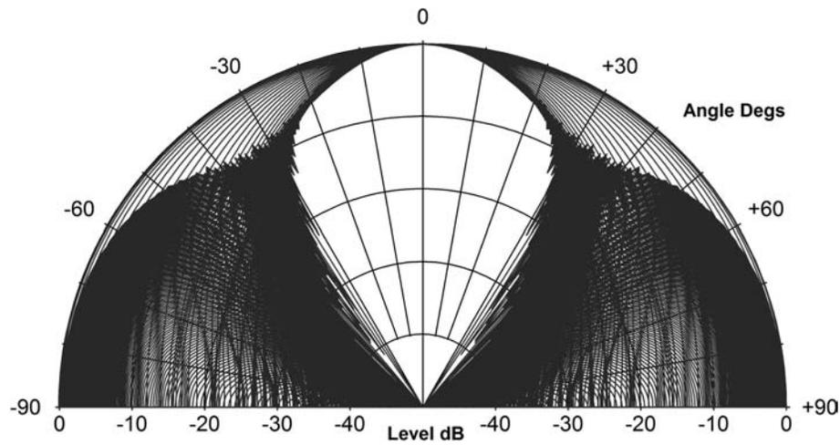
Fig. 22. Cylindrical composite polar plot for constant-beamwidth straight-line CBT array that provides a rounded-shape beam. Polar radial range is 50 dB with 10° angular increments.
