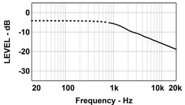
Fig. 16. Normalized far-field on-axis frequency response for circularly curved CBT constant-beamwidth array that provides a rounded-shape beam. Array maintains constant-beamwidth operation down to 800 Hz (—). The high-frequency power response of the CBT arrays rolls off at a rate of only 3 dB per octave, which is one-half of the 6 dB per octave rolloff rate of the previous constant-aperture arrays (Figs. 2 and 9).
