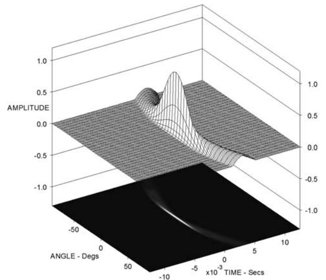
Fig. 20. Three-dimensional array coefficient plot versus frequency for constant-beamwidth curved-line CBT array. Note that plot does not include array's flat on-axis equalization and coefficients are independent of frequency.
