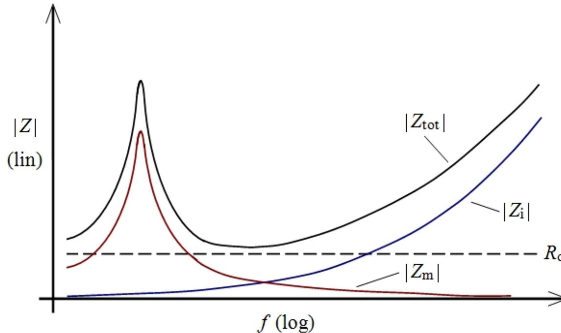
**Figure 2: Composition of the impedance magnitude curve of a typical cone driver. Both the motional impedance  $Z_m$  and the inductance impedance  $Z_i$  have considerable magnitude throughout the main operation area.**
