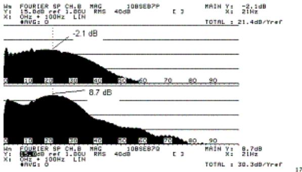
Figure 17: Sample 3: Ten Inches Speaker; Rubber Half Roll Surround. Frequency domain responses of the set with the voice coil glued to the cone. Comparison of the responses for two inputs at different levels
