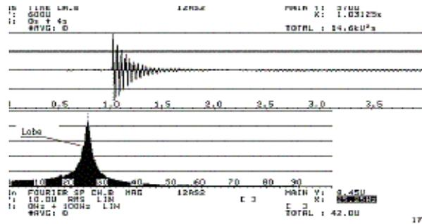
Figure 18: Sample 4: Twelve Inches Speaker; Foam, Half Roll Surround. Time signal and Fourier spectrum of the response for a medium level excitation (first positive time peak at 570 microns). Spectrum peak shows a small lobe on the peak left side
