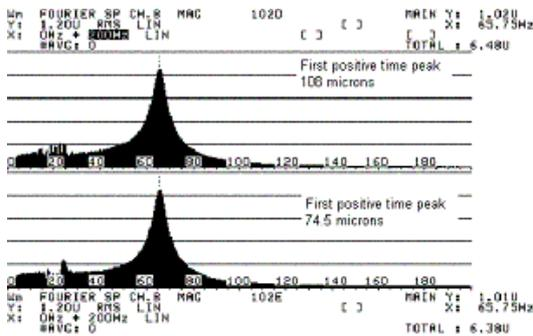
Figure 23: Sample 5: Ten Inches Speaker; Cloth Three Rolls (Accordion Type) Surround. Responses for two discrete excitations. The level of excitations was very small. First positive time peak for upper graph is 108 microns, and for the lower graph it is 74.5 microns. Notice the high repeatability and linear appearance
