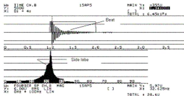
Figure 25: Sample 6: Fifteen Inches Speaker; Vulcanized Cloth Asymmetric Surround. Test for small - medium input force. Minimum negative time response at -355 microns Time window was extended to 1 second. Notice the modulation of the time signal (small beat) and the spectral consequence on the lobe at the left side of the spectrum peak
