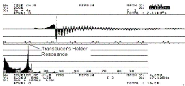
Figure 5: Time signal and Fourier Spectrum of the Transducer's Arm - Support Response to a mechanical pulse. The natural frequency of this transducer and arm at 17.125 Hz is clearly depicted
