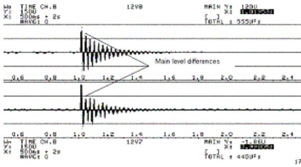
Figure 12: Sample 2: Twelve Inches Speaker; Cloth Three Rolls (Accordion Type) Surround. Time responses of the sample. The tests are low level type (max. peak is 120 microns). Test of response sensitivity to off center forces. The upper curve is the result of an applied force 6 mm at the right of the sample axis. The lower curve is the result of an applied force 6 mm at the left of the sample axis
