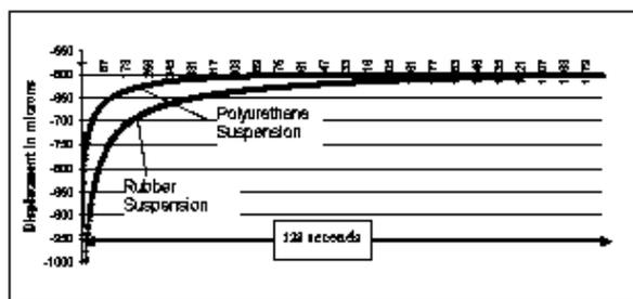
Figure 2: Displacement as a time function. Sudden release of two suspension – diaphragms, from 1mm from the measurement transducer to the rest position. Notice the slowness of the Rubber suspension sample going to the rest
