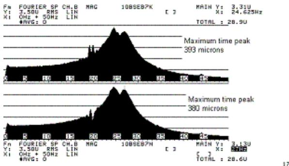
Figure 16: Sample 3: Ten Inches Speaker; Rubber Half Roll Surround. Frequency domain responses for two excitations of very similar input levels. Compare the results with those depicted in Figure 15. Notice the double peaks, or split peaks, and the differences between the two spectra
