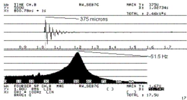
Figure 8: Sample 1: Ten Inches Speaker; Half Roll, Extra Wide (30mm diameter), Rubber Surround. Time signal and Fourier spectrum of the response, for a small – medium excitation level (first positive peak at 375 microns). Notice the shift of the eigenfrequency respect to Figure 7
