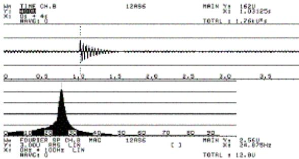
Figure 20: Sample 4: Twelve Inches Speaker; Foam Half Roll Surround. Time signal and Fourier Spectrum for small level of excitation, (first positive time peak at 162 microns). Spectrum peak is becoming asymmetric as input level decreases
