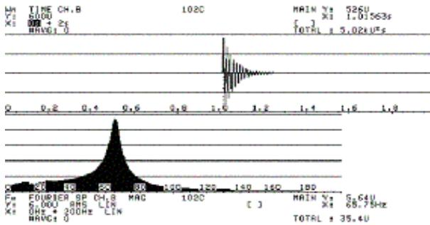
Figure 22: Sample 5: Ten Inches Speaker; Cloth Three Rolls (Accordion Type) Surround.- Test for a discrete medium level excitation. First positive time peak is 526 microns. Notice the remarkable linear appearance
