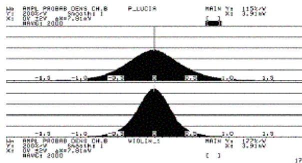
Figure 1: Amplitude Probability Density Function for two musical signals, showing the maximum values at zero amplitude. Upper figure is a Spanish guitar energetically played. Lower Figure is classical music, violin solo, gently played. Analyzer was set to the fastest sampling
