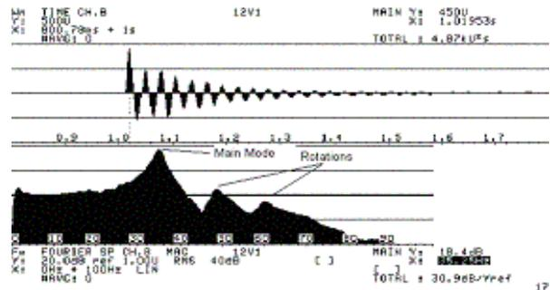
Figure 10: Sample 2:Twelve Inches Speaker; Cloth Three Rolls (Accordion Type) Surround. Time signal and Fourier spectrum of the response. Test at medium level excitation (first positive peak at 450 microns). Notice the secondary peaks the spectrum depicts
