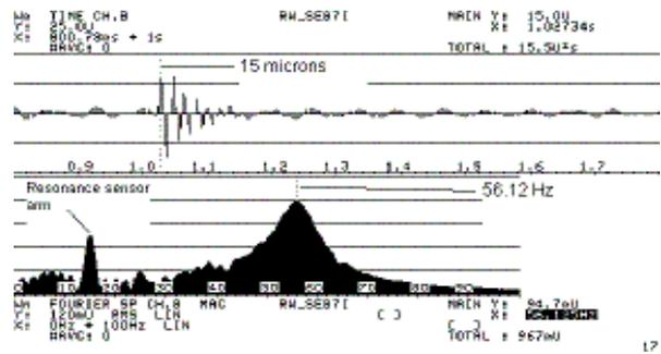
Figure 7: Sample 1: Ten Inches Speaker; Half Roll, Extra Wide (30mm diameter), Rubber Surround. Time signal and Fourier spectrum of the response for a very small force excitation. Maximum time response gives 15 microns
