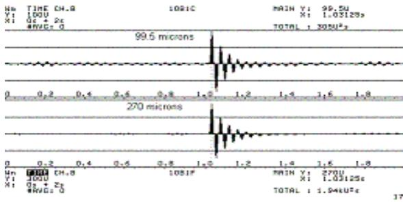
Figure 14: Sample 3: Ten Inches Speaker; Rubber Half Roll Surround. Time Domain responses. The test purpose is to compare the sample for inputs of different levels. The tested amplitudes are: very low level input force (max. peak is 99.5 microns) and low level (maximum peak is 270 microns)
