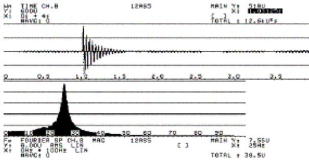
Figure 19: Sample 4: Twelve Inches Speaker; Foam Half Roll Surround. Time signal and Fourier spectrum of the response for a medium level excitation (first positive time peak at 518 microns). Spectrum contour is, almost, perfectly symmetric and smooth in the whole figure
