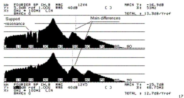
Figure 11: Sample 2: Twelve Inches Speaker; Cloth Three Rolls (Accordion Type) Surround. Fourier spectra of two responses. Test of repeatability for very small stroke. Upper and lower graphics have two different responses for the same input signal. The differences in the spectrum shape are in the secondary peak where the cursor is
