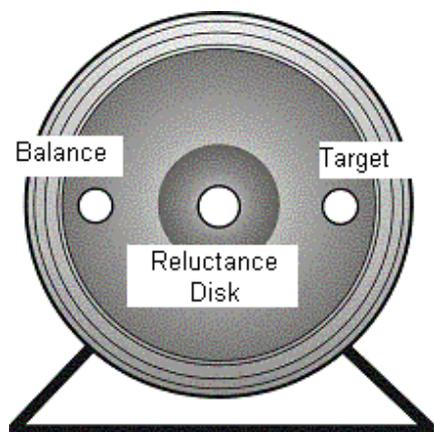
Figure 4: Detail of the target and balance disk, for the diaphragm response measurements by an Eddy current transducer. Notice disks are glued onto the diaphragm and close to the suspension. The high permeability disk for excitation, glued on dust cap, is also depicted
