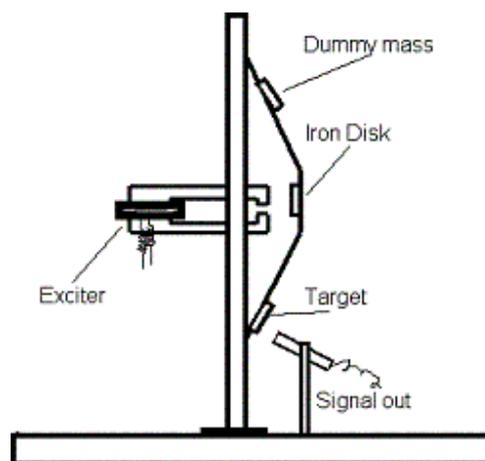
Figure 3: Test bench to evaluate the Suspension-Diaphragm performances. The lay out shows the exciting device, the receiver and the sample being tested
