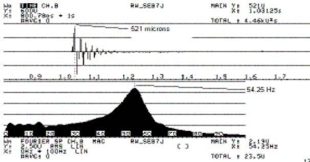
Figure 9: Sample 1: Ten Inches Speaker; Half Roll, Extra Wide (30mm diameter), Rubber Surround. Time signal and Fourier spectrum of the response for a medium excitation (first positive peak at 521 microns). Notice the shift of the eigenfrequency respect to Figures 7 and 8
