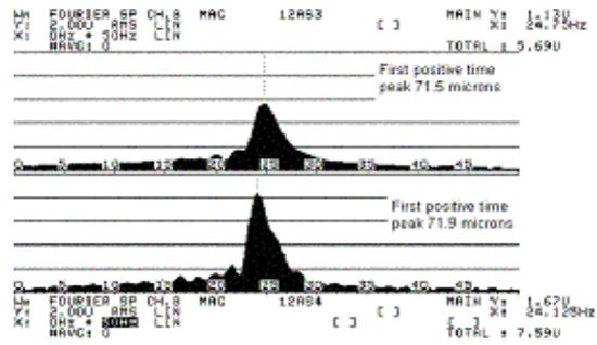
Figure 21: Sample 4: Twelve Inches Speaker; Foam Half Roll Surround. Fourier spectra of the responses for two discrete excitations of very small level. First positive time peak for the upper graph it is 71.5 microns; for the lower graph it is 71.9 microns. Notice the very low repeatability and nonlinear appearance
