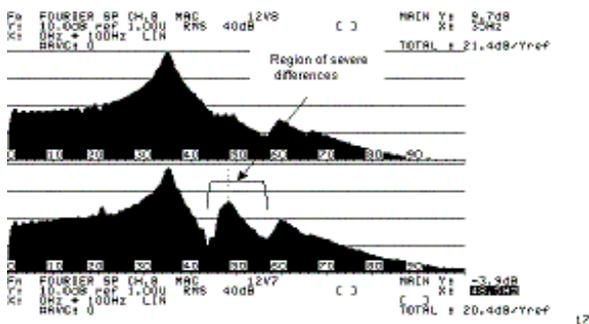
Figure 13: Sample 2: Twelve Inches Speaker; Cloth Three Rolls (Accordion Type) Surround. The graphs are Fourier Transforms of the time signals from Figure 12. Test is of low level type (max. peak is 120 microns). Upper graph depicts the spectrum response for a force applied 6mm to the right away from the axis of symmetry. Lower graph is the spectrum response for a force applied 6mm to the left from the axis of symmetry
