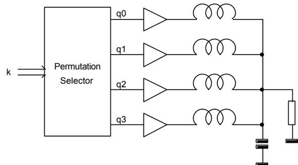
To control the unwanted circulating current in a sampled-time system, a measure of the circulating currents is obtained by digitally integrating the “voltage” (in reality the number of quanta) found across each inductor over sampled time. For a given data value  $k$ , the number of ways to arrive at this value is
