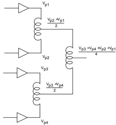
It can be seen that in this design, the multilevel signal will be physically present before the output filter.
