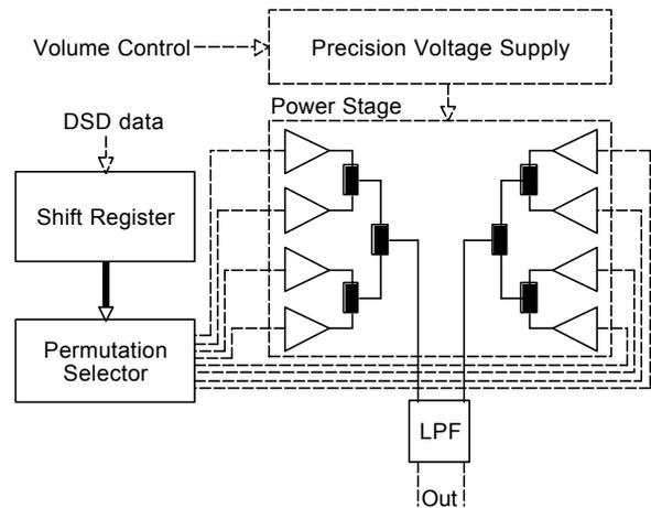
Each phase is a dual MOSFET in an SO-8 package together with a half-bridge driver, also in an SO-8. The switching rate is about 100kHz so the contribution of switching losses to heat dissipation may be neglected, counting only resistive losses. The on-resistance of the FETs is on the order of 150 mΩ (when hot). At a conservative rating of 1W per package the combined output current may be 10A<sub>rms</sub>. The power rating is 150W into 8Ω or 34.6V<sub>rms</sub>
