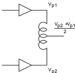
On the prototype, small toroids were used with the two winding halves bifilar wound to insure optimal coupling. The load current is shared between the two phases and will see only the leakage inductance of the coil (i.e. the magnetic fields caused by the two halves of the output current cancel out). A practical value of about 20nH is found. The inductance as seen between the two ends of the coil is
