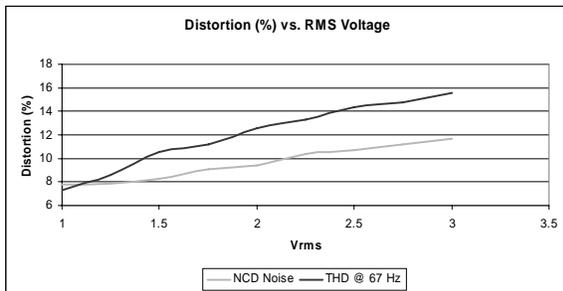
Figure 4: Loudspeaker Distortion vs. level
