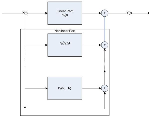
Figure 1: Equivalent Block Diagram of a Volterra Series
