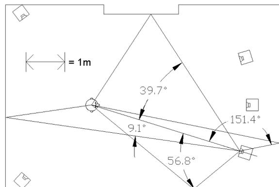
Fig. 6: Ray diagram for the right speaker of room 3 (a typical rectangular set-up).
