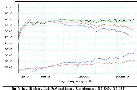
Fig. 13: Amplitude response of loudspeaker I.
