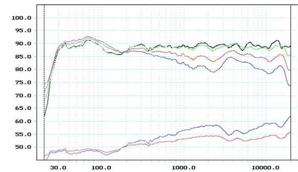
Fig. 15: Amplitude response of loudspeaker V.
