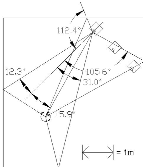
Fig. 7: Ray diagram for the left speaker of room 2 (a typical triangular set-up).
