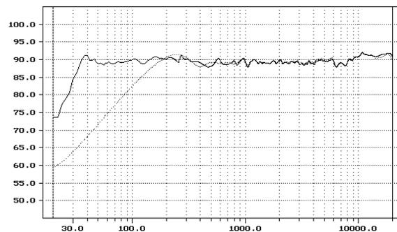
Fig. 1: On-axis amplitude response of a loudspeaker with a high Q resonance at 250Hz and a medium Q resonance at 600Hz. Solid: 500 ms gating, Dotted: 5 ms gating.
