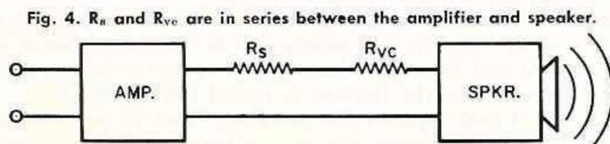
Fig. 4.  $R_s$  and  $R_{VC}$  are in series between the amplifier and speaker.
