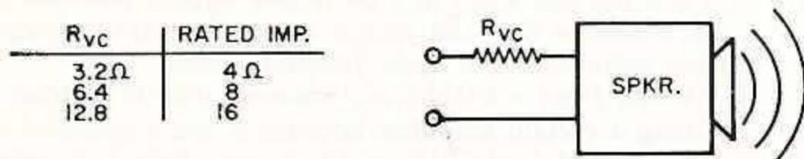
Fig. 3. Speaker resistance is about 80% of rated impedance.
