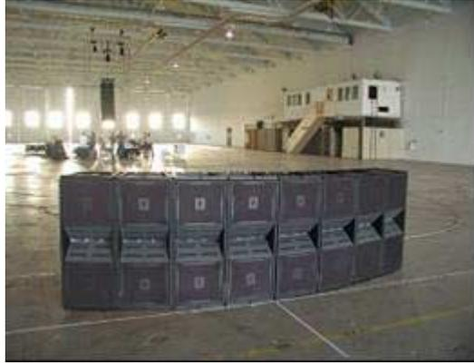
**Figure 44: Indoor ground plane setup for vertical polar response measurement of an eight element curved array.**
