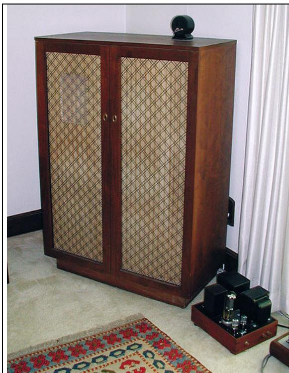
**Description:** Three-way, floorstanding loudspeaker with sealed-box woofer loading. Drive-units: eight 2" B-200Y Dual Treble aluminum-diaphragm tweeters, two 5¼" B-209B aluminum-cone midrange units, four 12" B-199A variable-density (pulp made from lambs' wool and shredded paper) cone woofers. Crossover: N-104 LC network. Crossover frequencies: 400Hz, 2.5kHz. Crossover slopes: 6dB/octave, first-order. Frequency range: 28Hz–20kHz. Nominal impedance: 8 ohms.
