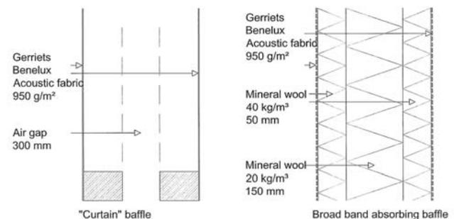
Figure 10. Baffle constructions for the ArenaA
