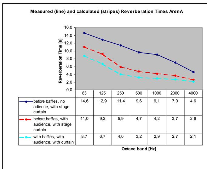
Figure 11. Measured (line) and calculated (stripes) RT's ArenA
