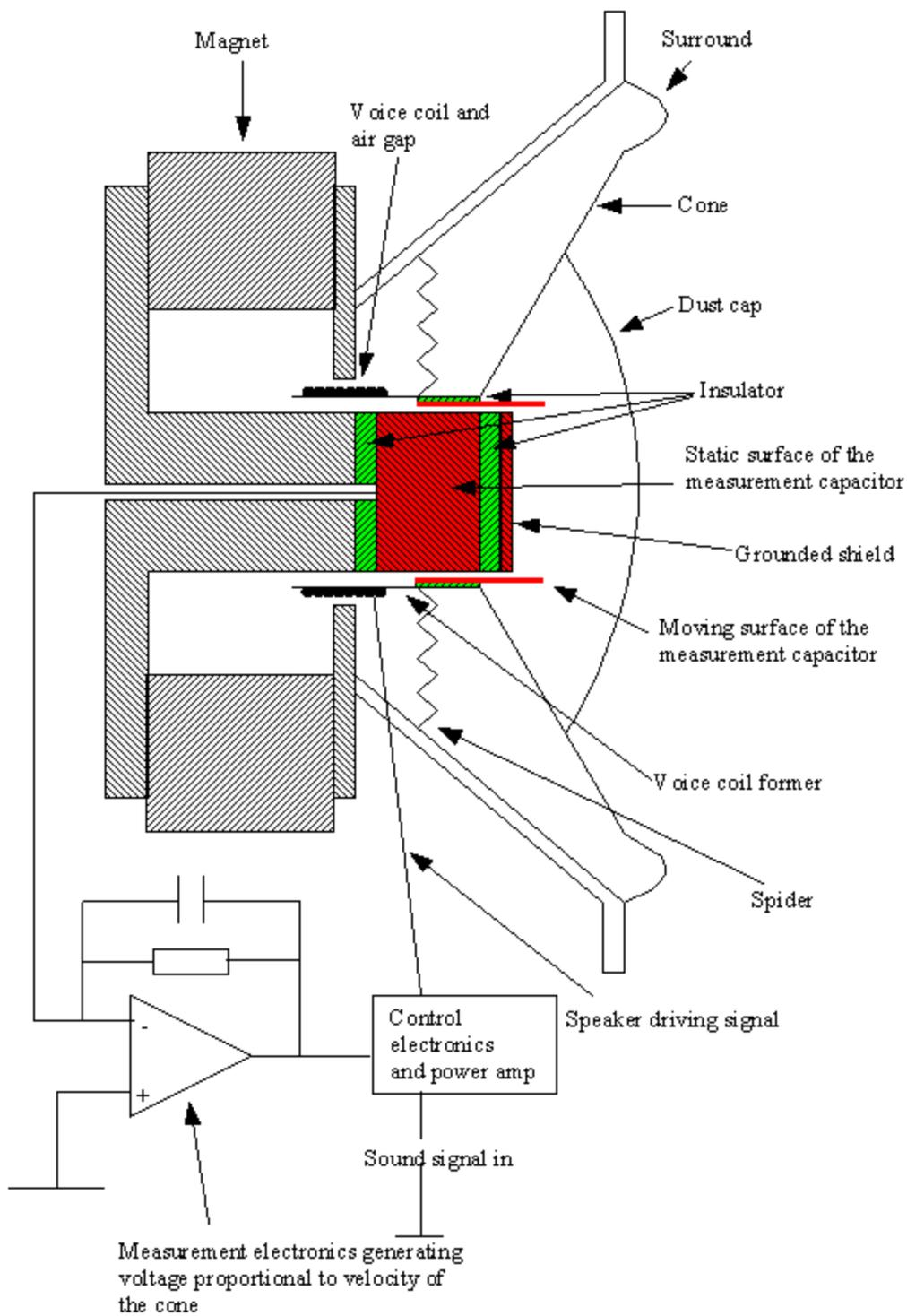
Figure 1: Principle of the measurement method
