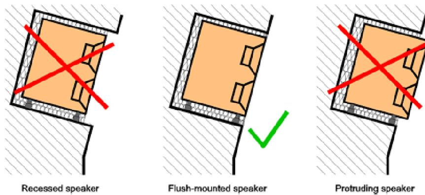
Figure 3. Flush-mounting a speaker correctly into a wall.
