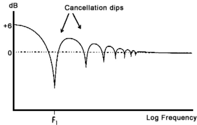
Figure 2. The frequency response dips caused by a wall reflection.
