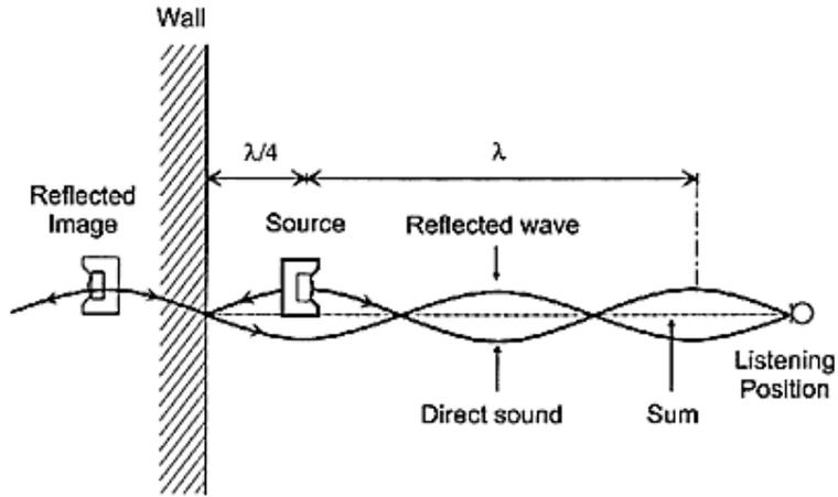
Figure 1. Sound reflection from a wall.
