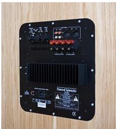
This rear panel of a powered subwoofer shows the heat sinks used to cool the power amplifier.
