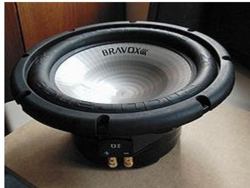
12-inch (30 cm) subwoofer driver (loudspeaker). A driver is commonly installed in an enclosure (often a wooden cabinet) to prevent the sound waves coming off the back to cancel out the sound waves being generated from the front of the subwoofer.
