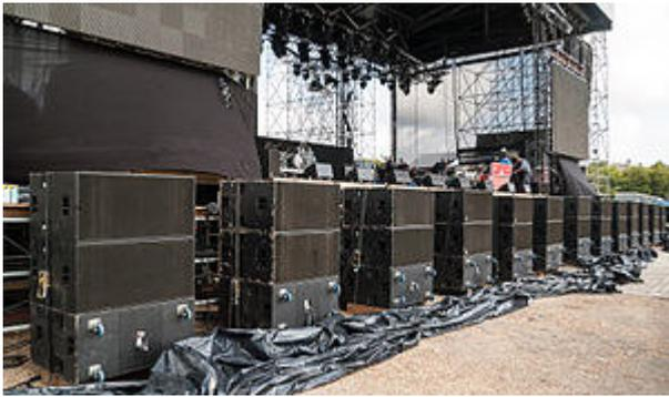
A row of subwoofer cabinets in front of the stage of a rock concert. One enclosure out of every stack of three is turned backward to make a cardioid output pattern.
