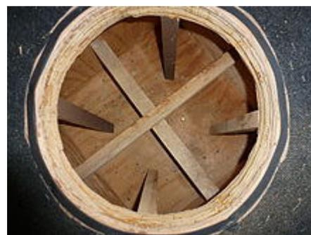
Heavily braced and built subwoofer enclosure
