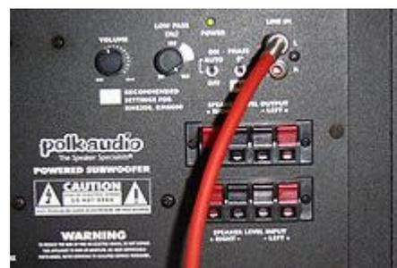
This picture of the rear panel of a Polk subwoofer cabinet shows a low-pass filter adjustment knob.
