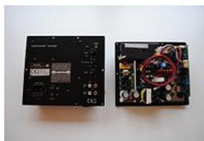
This picture of the internal components of an active (powered) subwoofer shows the circuitry for the power amplifier.
