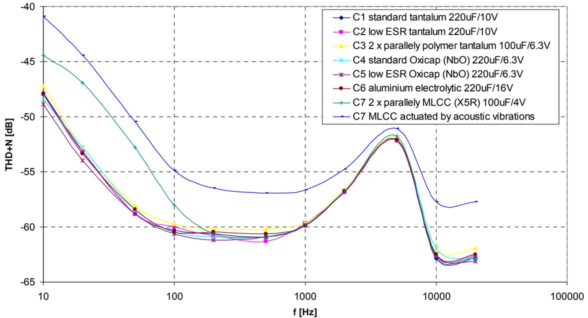
Figure 1: Harmonic distortion for different output coupling capacitors
