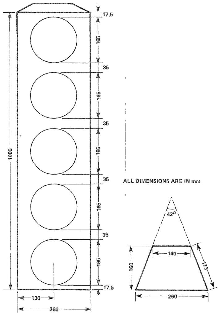
**Fig. 7** Cabinet details — all dimensions are in millimetres. The total cabinet volume is 0.324 cubic metres. A suitable material to use is 3/4" chipboard and this thickness needs to be added to the dimensions shown where appropriate.
