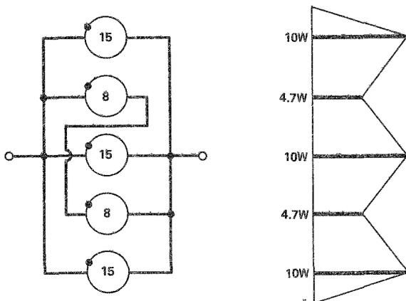
**Fig. 6** An alternative way to wire the speakers. This gives a power handling of nearly 40 W but is not recommended as the aperture is not correctly graded. The profile of the aperture is irregular, as shown.
