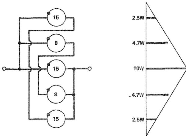
**Fig. 5** The wiring diagram for the 8 and 15 ohm speakers. Note how each speaker is wired in phase. For 10 W speaker units the power handling is about 25 W (actually 24.375 W). At right is shown the profile of the graded aperture.
