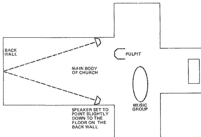
Fig. 8 The working layout of the speakers in the church.
