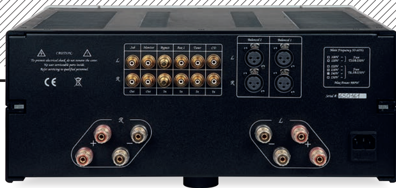
ABOVE: Six line inputs are provided (two balanced via XLRs) with two line outputs (monitor and subwoofer) alongside sets of 4mm bi-wire loudspeaker binding posts
